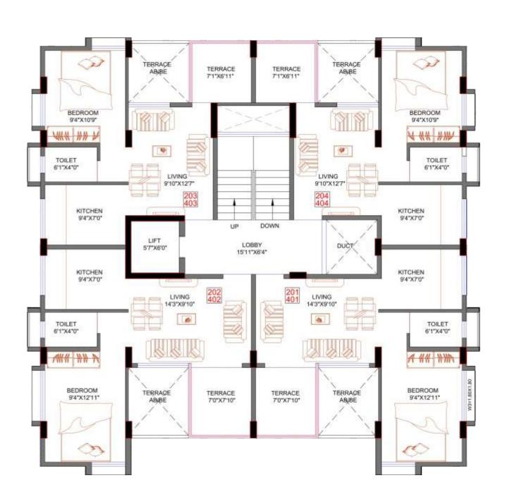
Typical Odd Floor Plan
